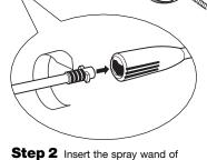
**Step 2** Insert the spray wand of your choice into the wand extension. Press in against the spring tension and twist into the locked position.
